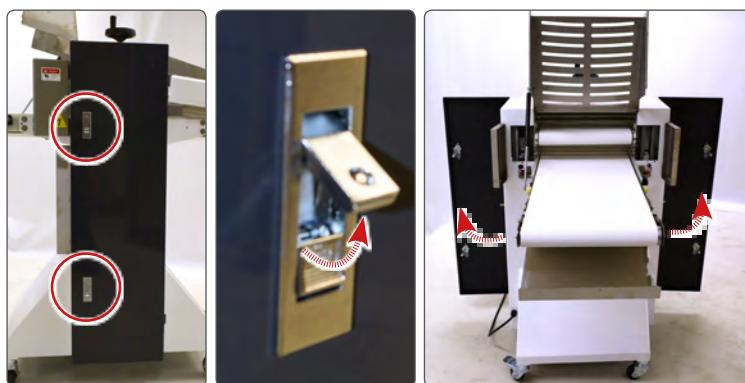
Unlock the push locks on the doors on both sides of the machine and open the doors.
