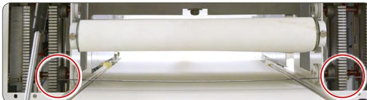
Check whether the blade is placed at the same height on both sides.
