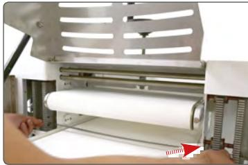
First slide the knife on 1 side of the blade holder into the blade slot at the desired height. (5 mm per slot) and then the other side.
