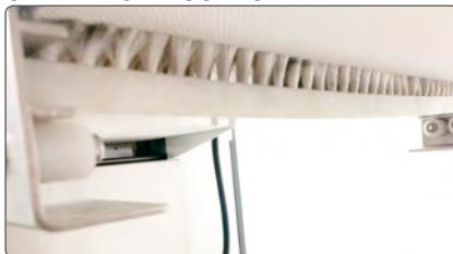
While the conveyor belt is running it passes the brush on the underside of the table.
