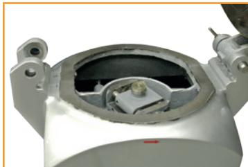
The moulding plate must be put back correctly. The slits in the base footing of the moulding plate have to fit upon the upper sliding faces of the side and the pin of the drive shaft has to fit into the ball bearing of the moulding plate.
